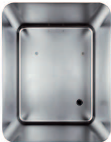
Detail of the inner chamber showing the position of the temperature probe and CO 2 sensor. On the lower right the standard access port is visible
