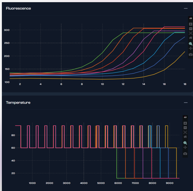
Fig 2: AutoNorm with iconPCR simplifies workflows and improves data quality. Users set a target amplification level, and each well stops cycling automatically once that level is reached. Shown is a dilution series of DNA libraries with fluorescence (top) and individual well temperatures (bottom) tracked in real time. High-concentration samples (green) reach the threshold first and enter a cold-hold phase, while lower-concentration wells continue cycling. Each sample stops precisely at the optimal point, with no manual intervention required.
