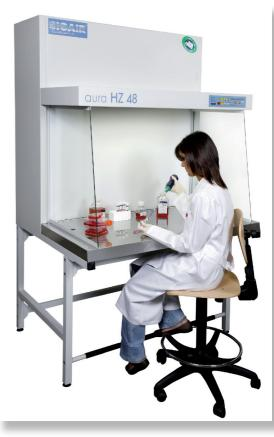
2. Lateral Flow Concept side walls: special tempered-glass side walls are installed inside the air flow, to prevent any leakage from the outside, thanks to the Venturi-effect.
