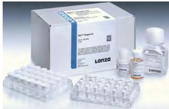
RAFT™ 3D Culture System consists of RAFT™ Reagent Kit and Absorbers for 96-well, 24-well or trans-well inserts.
