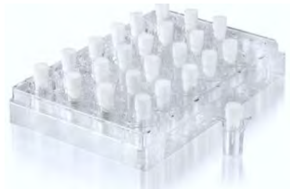
Absorbers being utilized with transwell inserts in a 24-well plate
