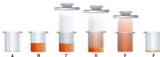
RAFT™ Sequence (A) Empty well or insert, (B) Cell and collagen mix forms hydrogel at 37°C, (C) Absorber contacts the hydrogel, (D) Liquid starts to be absorbed, (E) Process concentrates cells and collagen, (F) In less than 1 hour culture formation complete.
