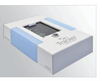
The high-end Micronic Tracxer Code Reader RD235 CRYO reads whole racks filled with 2D Data-Matrix or TraXis coded tubes. The reader features a CCD image sensor ensuring the highest accuracy 2D code reading, and an anti-frost system so that tube codes from even frozen samples can be read.
