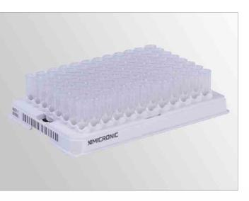
The Loborack-96 and Roborack-96 are based on the global recognized ANSI / SLAS standards for storage racks, feature a laser etched 1D rack barcode on one side of the rack and 'Twist-Lock' to prevent tubes from turning during screw (de)capping.
