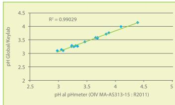
ANALYSIS EXECUTED THROUGH PH METHOD HAVE BEEN COMPARED AND CORRELATED WITH THE VALUES DETERMINED BY GLOBAL 240 AND KEYLAB ANALYZERS.
