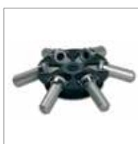
6 x 5 mL swing-out rotor (Cat. No. CC480138)
