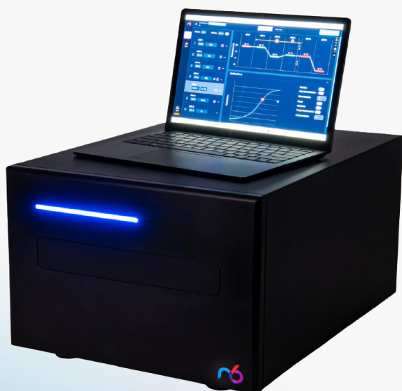
Figure 1. iconPCR, the world's first real-time thermocycler with 96 individually controlled wells.
