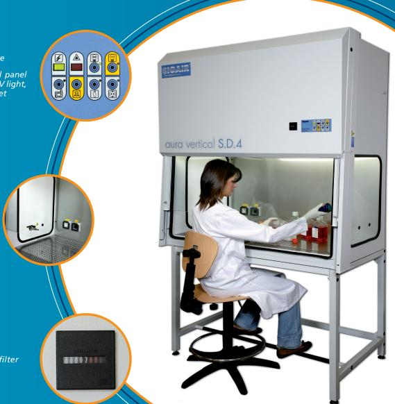
Aura Vertical S.D.4 is a partial-recirculating Class 100 vertical laminar airflow: air coming through the front aperture is mixed underneath the work surface with the downflow air and recirculated.
