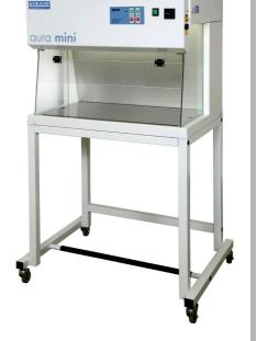
OUTWARD air barrier. In this case the air is sucked through the Filtrete® prefilter, mixed with the incoming recirculating air and then filtered through the main HEPA filter into the work area: here 30% of the air is exhausted through the front opening and 70% is recirculated. This configuration ensures the highest product protection.
